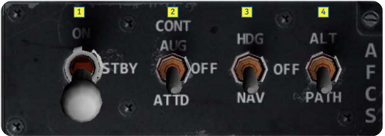
The automatic flight control system (AFCS) is a three axis autopilot. There are basically five operational modes provided by the AFCS:
