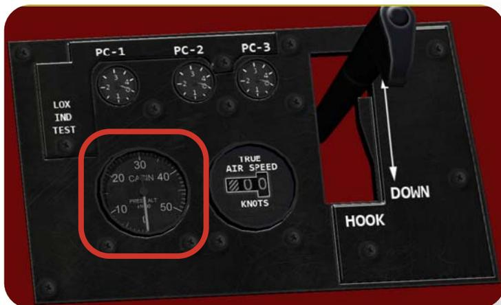
The cockpit is unpressurized from sea level to 8,000 feet. From 8,000 feet to 23,000 feet the regulator maintains a cockpit pressure equivalent to 8,000 feet. Above 23,000 feet, the regulator maintains a 5.0 psi pressure differential between cockpit and flight altitude pressures. At flight altitude of 50,000 feet, the cockpit pressure is about 20,000 feet.
