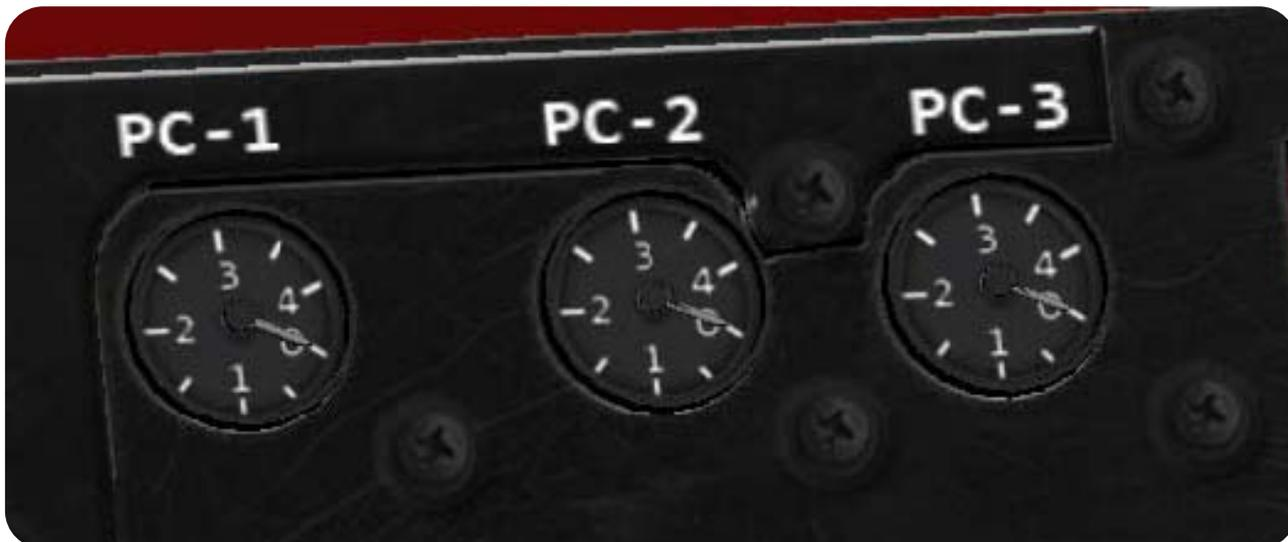
Hydraulic power is supplied by three independent systems: PC-1, PC-2 and PC-3. Each system is operated by an independent pump and operates at 3,100 psi. The Emergency Power Package (EPP) hydraulic pump supplies emergency power to the PC-1 and PC-3 systems.
